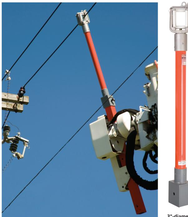
3"-diameter Epoxiglas<sup>®</sup> Jib Extension with Wireholder PST4002818
