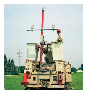
For armless construction, shorter crossarm mounts midway with single wireholder at top of mast. Notice, too, that center wireholder may be used alone for singlephase lifts.
