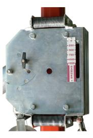
A scale on each side of monitor displays constant readout of load uplift for easy visibility from both buckets.
