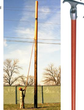
When space is extremely limited for truck storage, a 23 ft. Telescoping Tool that compacts to 4 ft. is available as Catalog No. C4031739.
