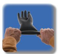
2 Stretch to seal closed Mechanical Inflators ASTM F 1236 maximum inflation limits: • Type I 2 times normal size • Type II 11/4 times normal size
