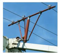
For three phase applications. The auxiliary arm may be rotated to align the wire holders with the conductors, then locked in position.
