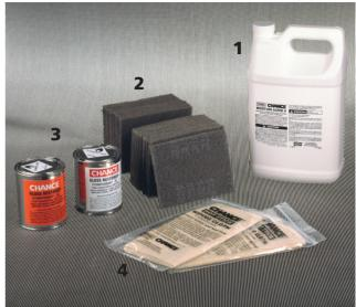
4. Hot Stick Wiping Cloths — Silicone impregnated cloths are used to wipe down mildly contaminated Epoxiglas, removing dust and dirt, and depositing a thin protective film on the surface of the tool. They give an added measure of protection when used after recoating with gloss restorer
